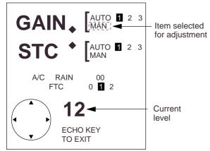
Figure 5-14 Display for adjustment of gain, STC, A/C RAIN and FTC
